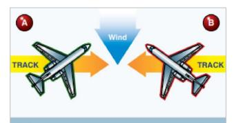
Traffic information would be issued to the pilot of aircraft "A" as 12 o'clock. The actual position of the traffic as seen by the pilot of aircraft "A" would be 1 o'clock. Traffic information issued to aircraft "B" would also be given as 12 o'clock, but in this case, the pilot of "B" would see traffic at 10 o'clock.
