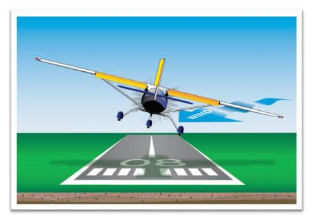
**Ground loop** Sideloads and/or improper wind correction may cause lose of control
